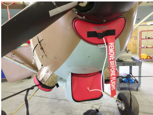
Siai Marchetti 1019 Engine Plugs, Prop Tie-Exhaust Covers
