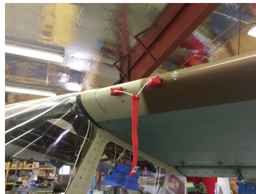
ENGINE PLUGS PREVENT BIRD NEST FOD. Piper Saratoga Engine Cowling Bird's Siai Marchetti 1019 Ventilation Scoop Plugs Nest
