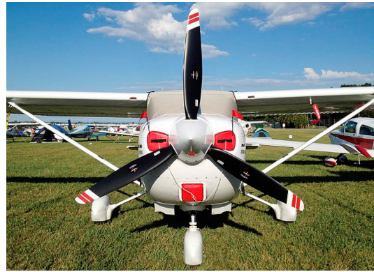
Cessna 182 S-model Engine Inlet Plugs (Including inlet plugs and third induction plug)
