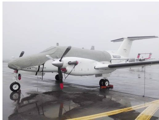
King Air 200 Canopy/Nose Cover, Engine Plugs & Prop Ties
