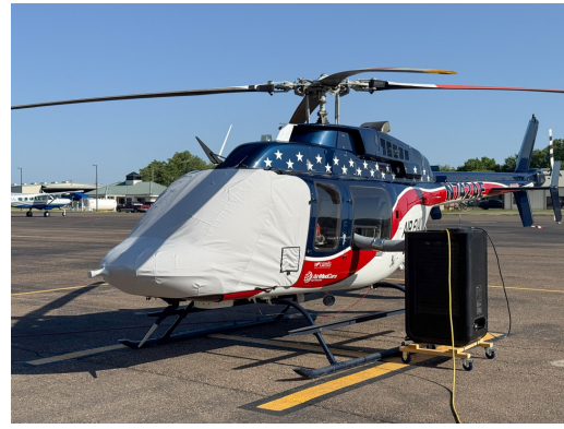
Bell 407 Abbreviated Bubble Cover, secures to front doors.
