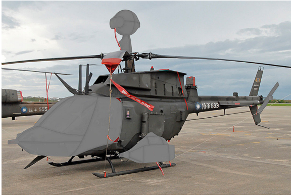
Windshield/Nose, Mast Antenna, 50 Cal, ALQ & Tail Rotor Covers
