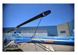
Bell 206B Jetranger (OH58, TH-57) Blade Covers, Van Horn Aviation Composite Blade
