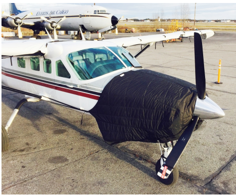
Cessna 208 Caravan Insulated Engine Cover, fully enclosed
