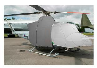
Forward Cabin Nose & Mid-Cabin/Engine Cover (extended to cross tubes)
