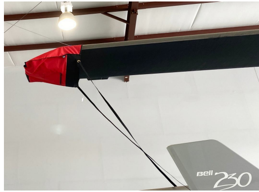
Bell 230 Blade Tie-Downs, (Semi-Rigid) W/Telescoping Attachment Handle
