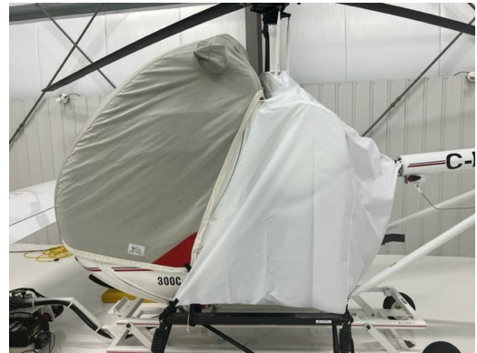
Schweizer 300C Engine Cover, test fit cover
