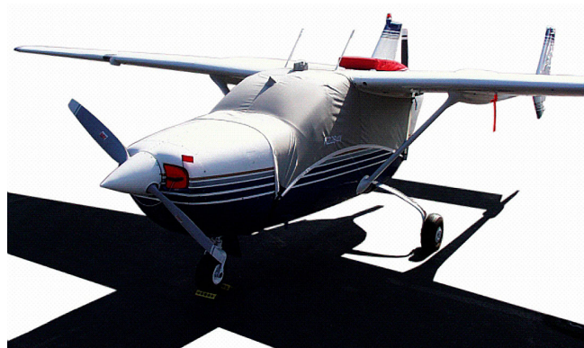
Cessna Skymaster Canopy Cover with Forward Extension, Fwd. Engine Plugs, Aft Engine Cover
