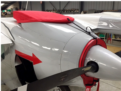
Cessna 337 Skymaster Aft Engine Inlet Cover, hoop type, & outlet plugs (SOLD SEPARATELY)
