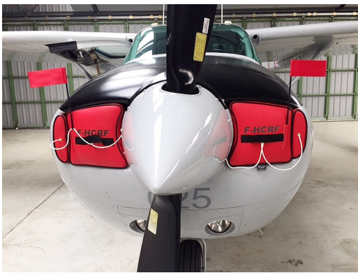
Cessna 337 Skymaster Forward Engine Inlet Plugs
