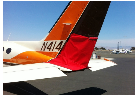
Cessna 414 Rudder Openings Cover (bird barrier)
