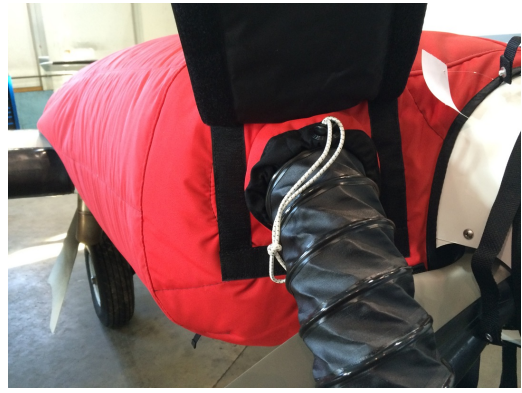
Cessna 402 Insulated Engine Cover with Heater
