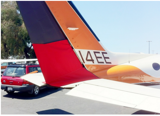
Cessna 414 Rudder Openings Cover (bird barrier)
