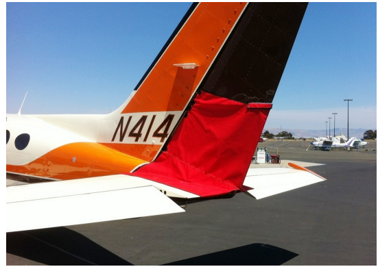
Cessna 414 Rudder Openings Cover (bird barrier)
