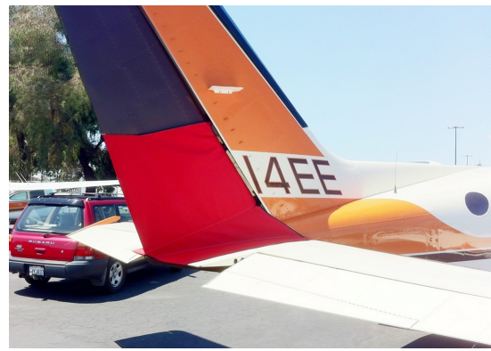
Cessna 414 Rudder Openings Cover (bird barrier)
