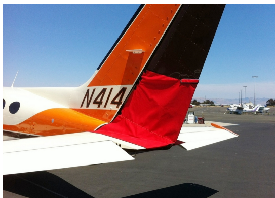
Cessna 414 Rudder Openings Cover (bird barrier)
