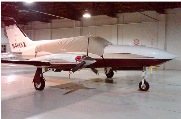
Cessna 414 Canopy Cover and Engine Inlet Plugs
