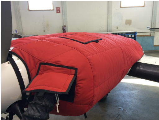
Cessna 402 Insulated Engine Cover with Heater
