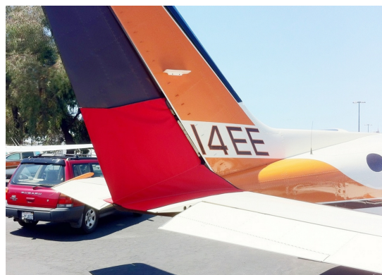
Cessna 414 Rudder Openings Cover (bird barrier)
