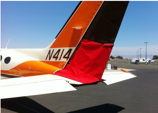
Cessna 414 Rudder Openings Cover (bird barrier)
