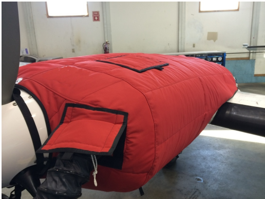
Cessna 402 Insulated Engine Cover with Heater
