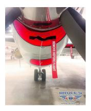
**Engine and Oil Cooler Inlet Plugs**
