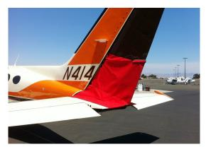
Cessna 414 Rudder Openings Cover (bird barrier)
