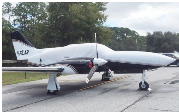
Cessna 421 Canopy Cover, Engine Plugs
