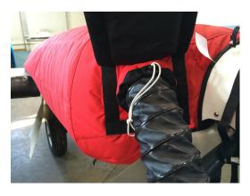
Cessna 402 Insulated Engine Cover with Heater
