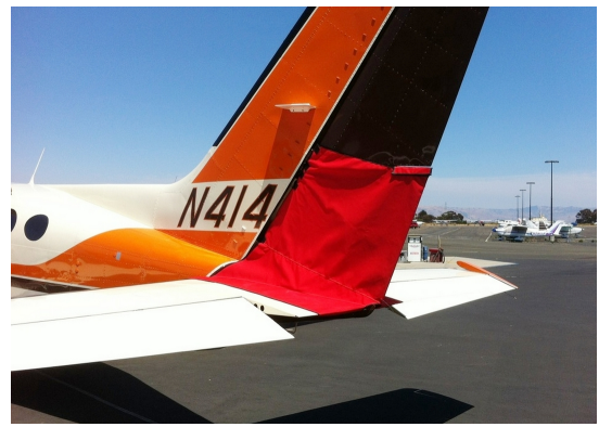
Cessna 414 Rudder Openings Cover (bird barrier)
