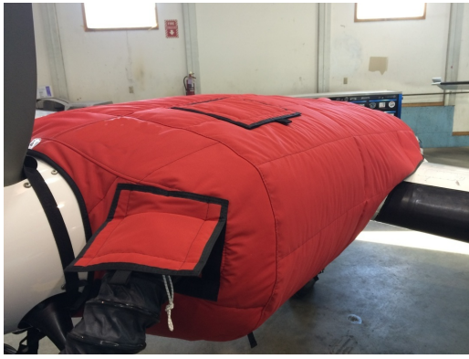
Cessna 402 Insulated Engine Cover with Heater
