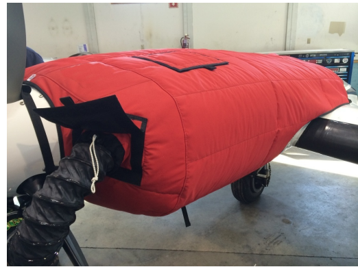
Cessna 402 Insulated Engine Cover with Heater
