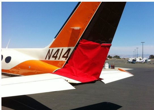
Cessna 414 Rudder Openings Cover (bird barrier)
