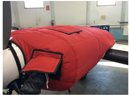
Cessna 402 Insulated Engine Cover with Heater
