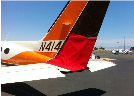
Cessna 414 Rudder Openings Cover (bird barrier)
