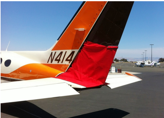
Cessna 414 Rudder Openings Cover (bird barrier)
