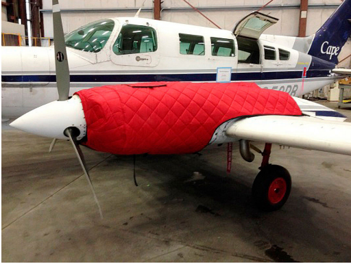
Cessna 402 Insulated Engine Cover
