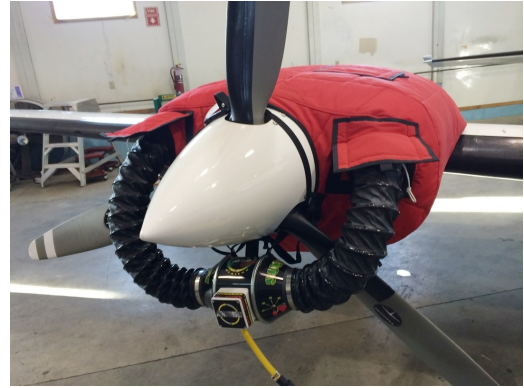
Cessna 402 Insulated Engine Cover with Heater
