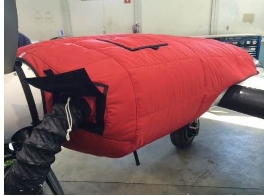
Cessna 402 Insulated Engine Cover with Heater
