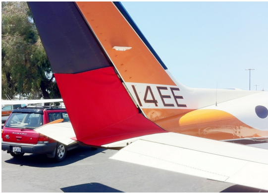
Cessna 414 Rudder Openings Cover (bird barrier)
