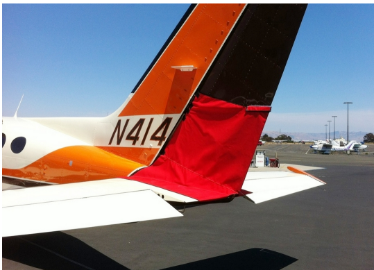
Cessna 414 Rudder Openings Cover (bird barrier)
