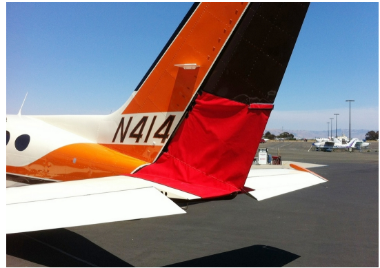
Cessna 414 Rudder Openings Cover (bird barrier)
