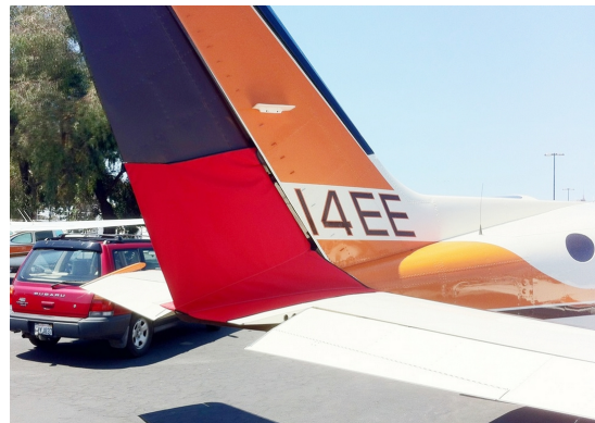
Cessna 414 Rudder Openings Cover (bird barrier)
