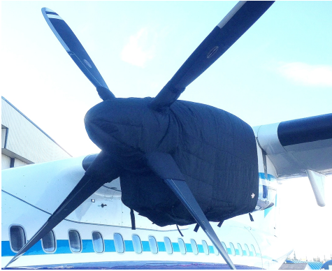
ATR-72-202 Insulated Engine & Prop Hub Covers
