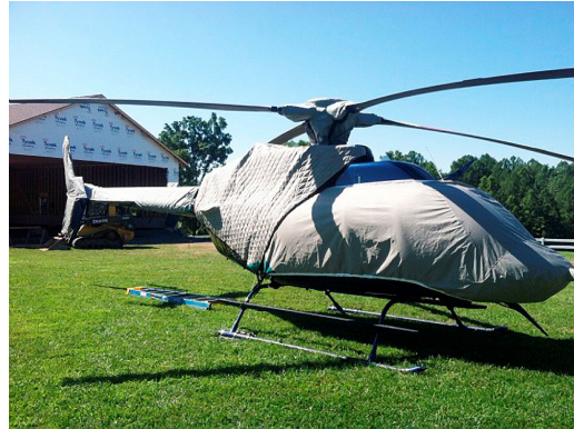
Bell 407 Covers: Bubble, Insulated Engine, Rotor Mast, Blades, Tailboom, Vertical Stabilizer and Tail Rotor
