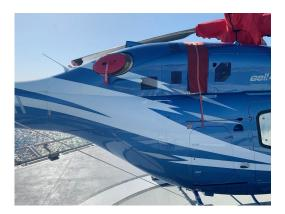
Bell 429 Exhaust Plug, Rotor Mast Cover
