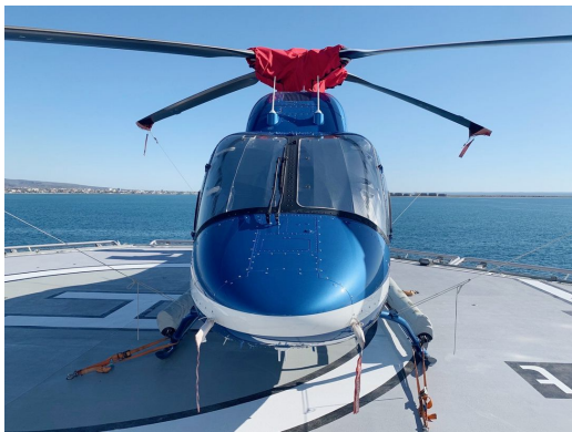
Bell 429 Windshield HeatShields, Rotor Mast Cover
