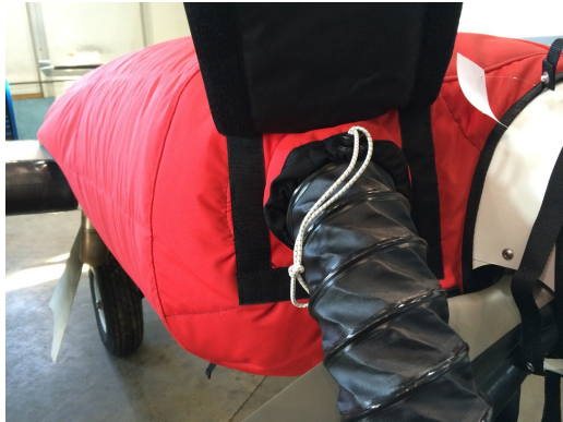
Cessna 402 Insulated Engine Cover with Heater
