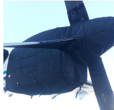
ATR-72-202 Insulated Engine & Prop Hub Covers
