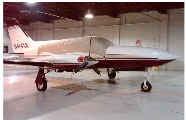
Cessna 414 Canopy Cover and Engine Inlet Plugs
