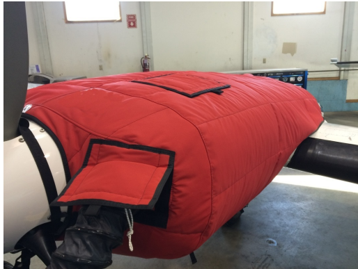
Cessna 402 Insulated Engine Cover with Heater
