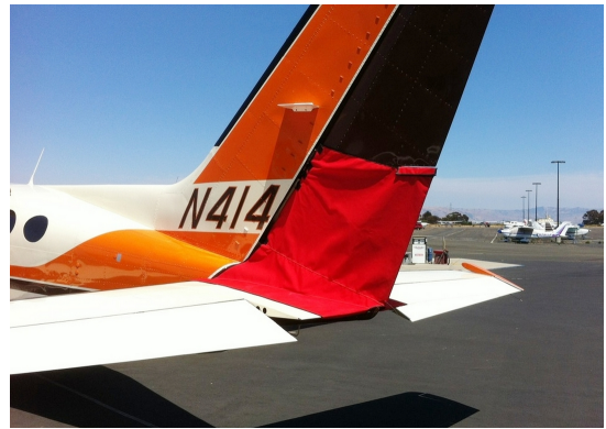
Cessna 414 Rudder Openings Cover (bird barrier)
