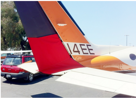
Cessna 414 Rudder Openings Cover (bird barrier)
