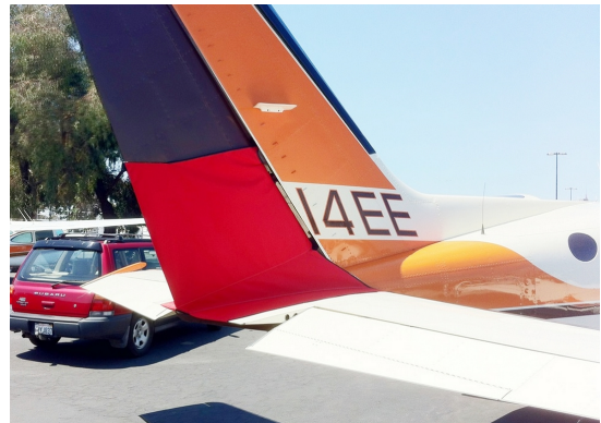
Cessna 414 Rudder Openings Cover (bird barrier)
