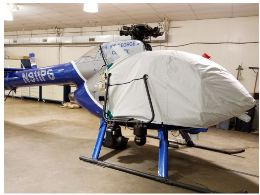
McDonnell Douglas MDD 520 Notar Bubble Cover, with special missions equipment.
