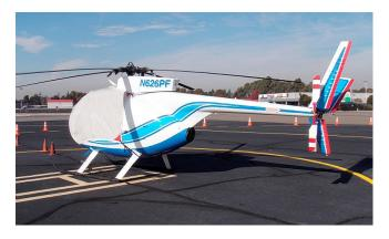
Hughes 500D Bubble Cover with Wire Strike detail and Blade Tie-downs
