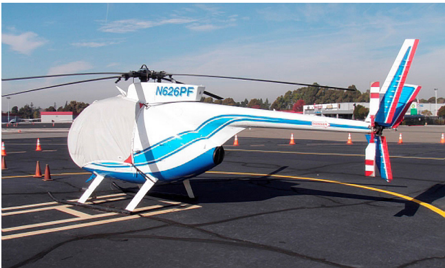
MD500C Bubble Cover with Wire Strike detail
