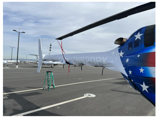
Bell 505 Tailboom & Stabilizer Covers, test fit cover
