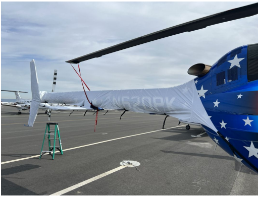
Bell 505 Tailboom & Stabilizer Covers, test fit cover
