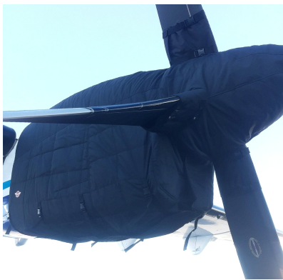
ATR-72-202 Insulated Engine & Prop Hub Covers
