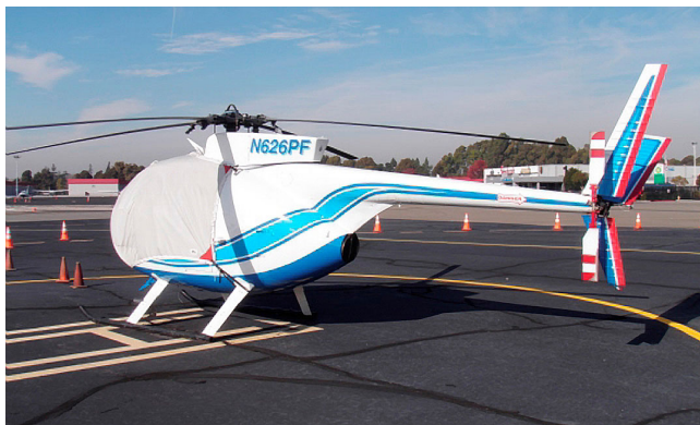
MD500C Bubble Cover with Wire Strike detail
