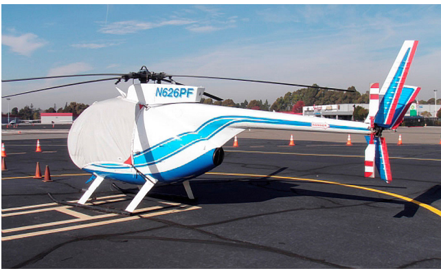
MD500C Bubble Cover with Wire Strike detail
