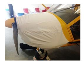
A-22 Engine Cover, test fit
