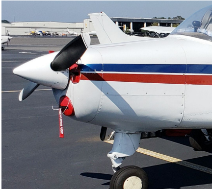
Beech Musketeer Engine Inlet Plugs ENGINE PLUGS PREVENT BIRD NEST FOD. Piper Saratoga Engine Cowling Bird's Nest
