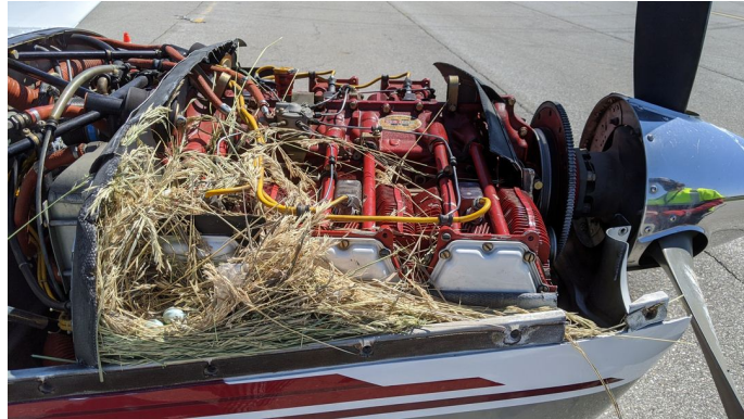
Beech Musketeer Engine Inlet Plugs ENGINE PLUGS PREVENT BIRD NEST FOD. Piper Saratoga Engine Cowling Bird's Nest
