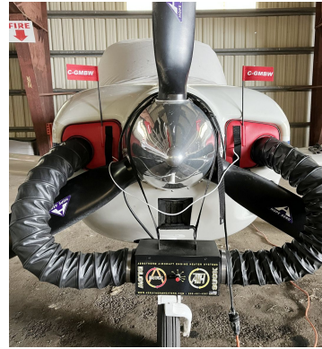
Beech Sierra Engine Inlet Plugs w/ Aerotherm Heater Openings
