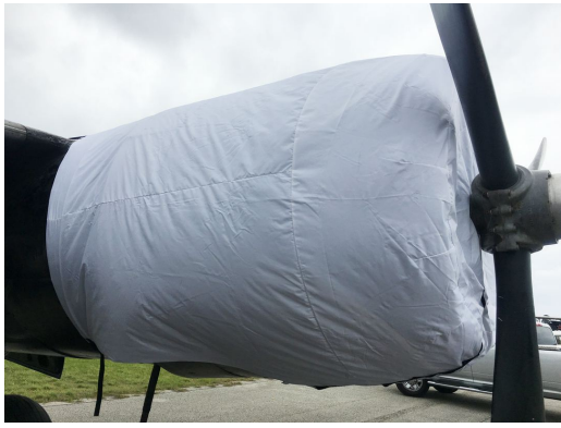
Douglas A-26 Engine Cover, test fit cover
