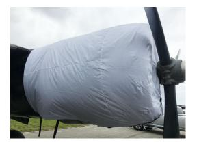
Douglas A-26 Engine Cover, test fit cover
