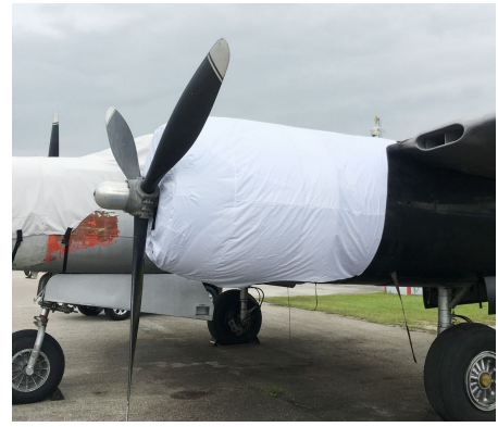
Douglas A-26 Engine Cover, test fit cover
