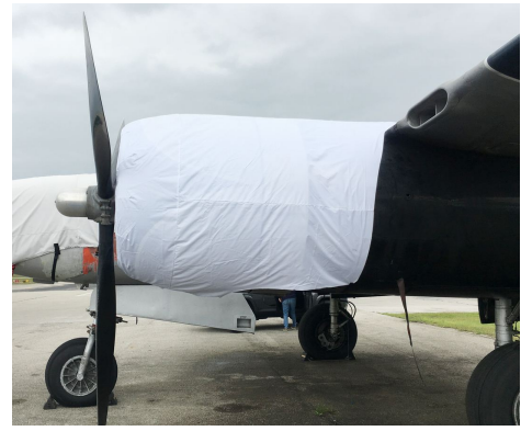
Douglas A-26 Engine Cover, test fit cover
