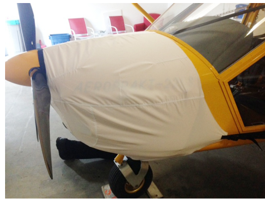
A-22 Engine Cover, test fit
