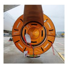
Airbus A320 Exhaust & Bypass Vent Plugs
