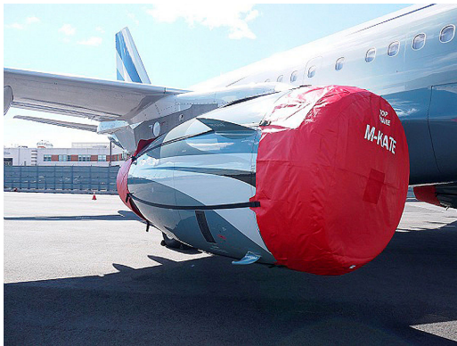
Airbus A319 Intake/Exhaust Covers set, IAE V2500
