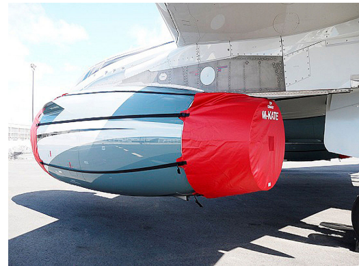
Airbus A319 Intake/Exhaust Covers set, IAE V2500
