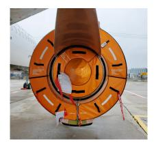
Airbus A320 Exhaust & Bypass Vent Plugs
