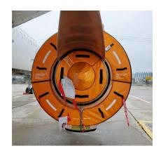
Airbus A320 Exhaust & Bypass Vent Plugs
