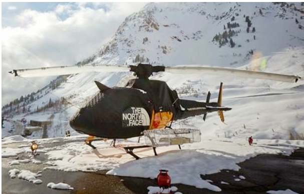
AS350 Insulated Bubble, Engine & Rotor Hub Covers Bubble Cover, Intake/Exhaust, Rotor Mast, Tail Rotor & Main Body Covers
