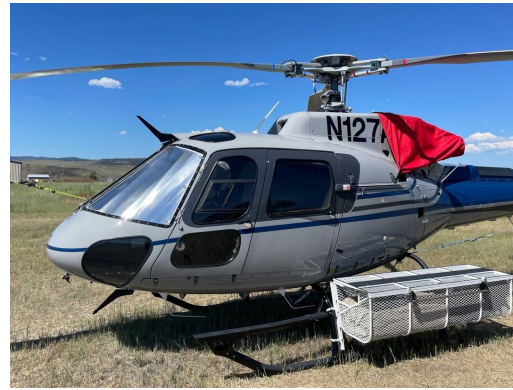
Eurocopter AS350-B3 Cabin HeatShields, Intake/Exhaust Cover
