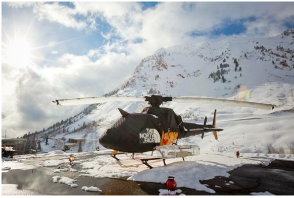
AS350 Insulated Bubble, Engine & Rotor Hub Covers
