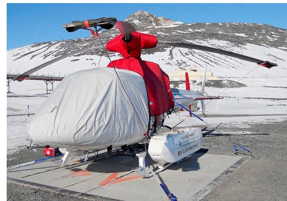
AS350 Bubble Cover w/ Cargo Mirror, Blade Tie-downs, Insulated Engine, Insulated Main Rotor Hub and Insulated Tail Rotor Covers
