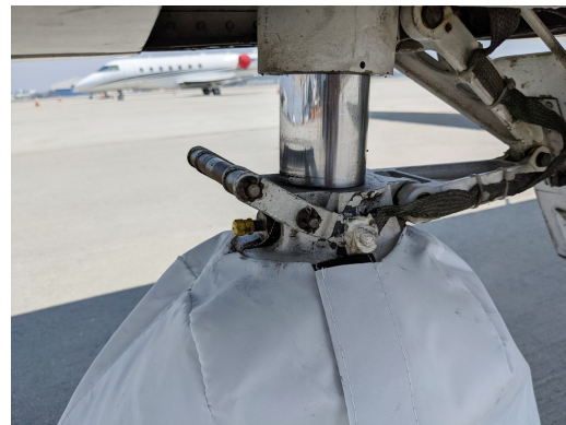
CJ1 Nose Gear Tire Cover, test fit
