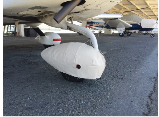
Grumman AA5 Nose Wheelpant Cover, test fit
