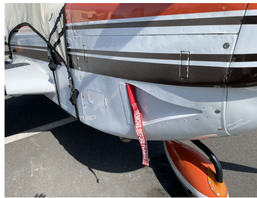
Grumman AA5 Side Cowling Inlet Plug
