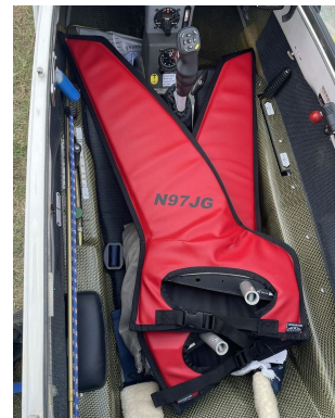
Schempp-Hirth Ventus-2B winglet/wingtip pads
