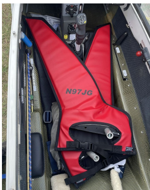
Schempp-Hirth Ventus-2B winglet/wingtip pads
