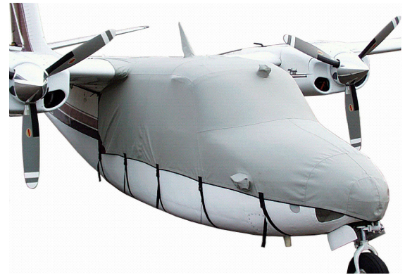
Canopy/Nose Cover (extends over top past leading edge)
