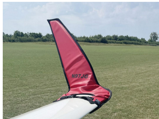
Schempp-Hirth Ventus-2B winglet/wingtip pads
