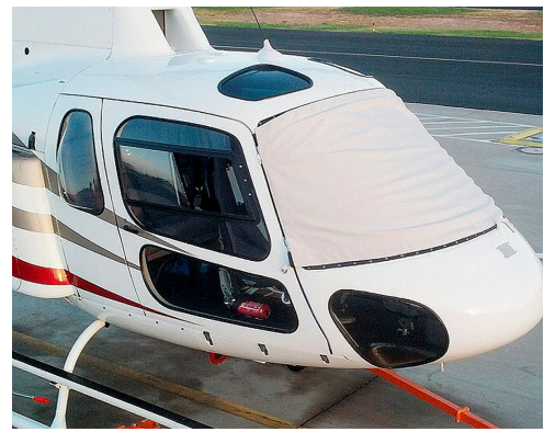
AS350 Windshield Cover, pinches in door jambs
