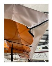
Aeromarine Merlin Horizontal Stabilizer Covers, test fit covers
