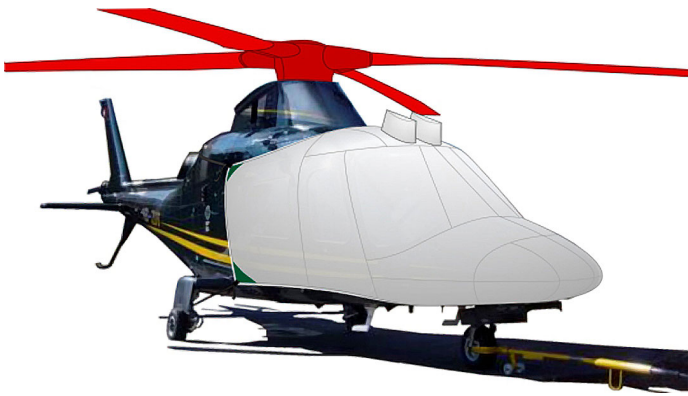
Agusta 109 Bubble, Rotor Hub & Blade Covers (illustration)
