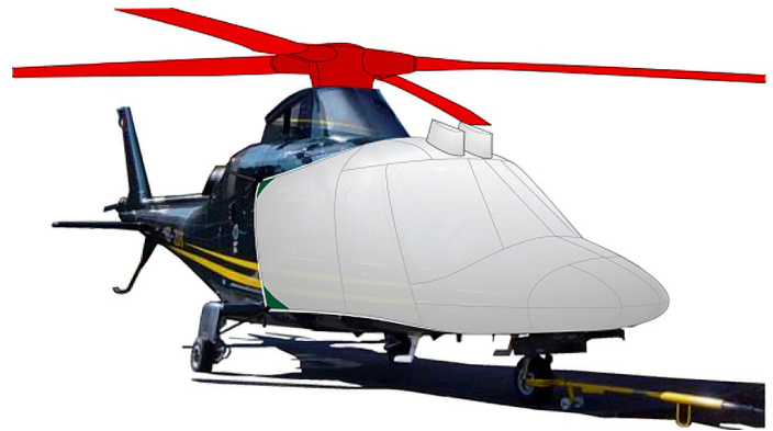
Agusta 109 Bubble, Rotor Hub & Blade Covers (illustration)
