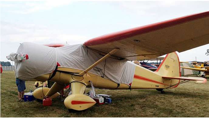
Stinson Reliant Over-the-top Canopy, Engine & Propellor Covers
