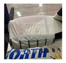
ATR-42-300 Insulated Engine Cover, test fit cover
