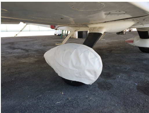
Grumman AA5 Main Wheelpant Cover, test fit
