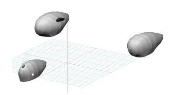
Grumman AA5 Wheelpant Covers, 3D model
