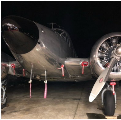
Beech 18 Engine & Oil Cooler Inlet Plugs
