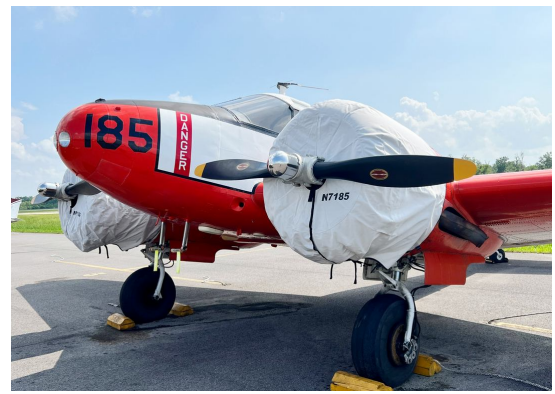
Beech 18 Engine Covers, non-insulated
