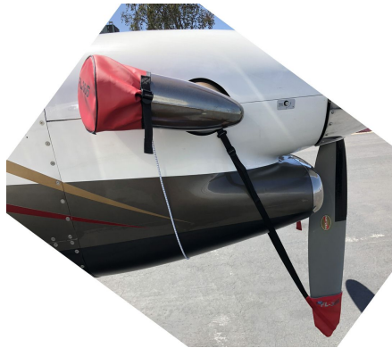
Beech King Air 350 Prop Tie-Downs/Exhaust Covers Combination
