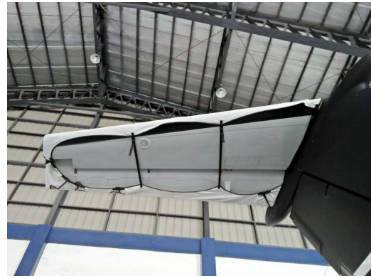
Beech King Air B350 Horizontal Stabilizer Covers
